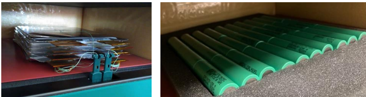
Fig. 1. left: Pouch cells stacked in HFM; right: Cylindric lithium-ion battery cells in HFM
