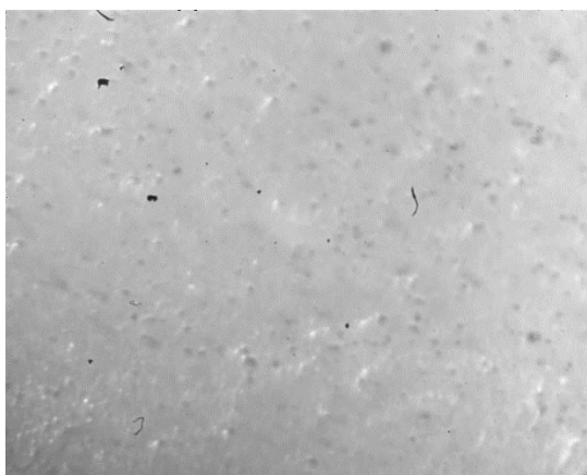
Fig. 1. Liquid-Liquid Equilibrium observed in a dark oil under high pressure with the full visibility setup equipped with a SWIR camera
