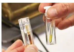
Figure 1. Two ampoules containing a reactive mixture composed by N_2O_4 and NO_2 , and following the reaction N_2O_4 = 2 NO_2 according to chemical equilibrium. The ampoule on the left is at higher temperature and thus contains mostly NO_2 , the ampoule on the right is at lower temperature and thus contains mostly N_2O_4 .
